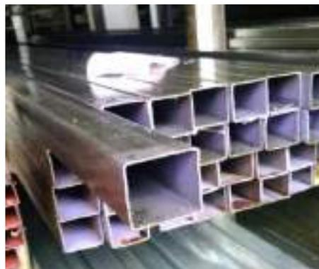
**Gambar 3. 18** Besi *hollow square* 40 x 40 mm
