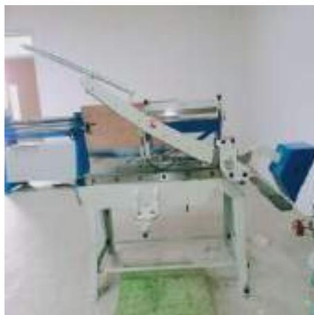
**Gambar 3. 2** Mesin *shearing*
