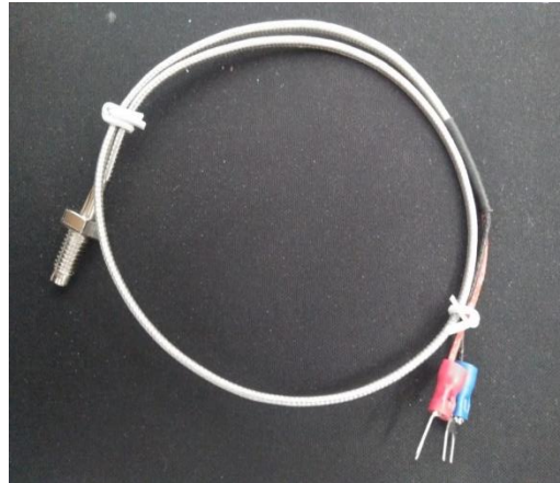
Gambar 2.2 Sensor suhu termokopel tipe-K
