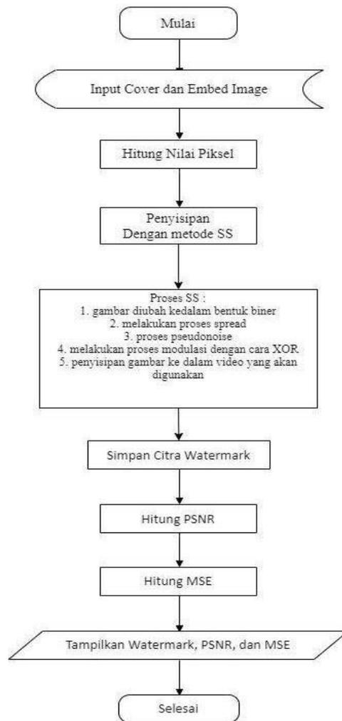
**Gambar 3.7** Flow Chart Proses Penyisipan Metode Spread Spectrum
