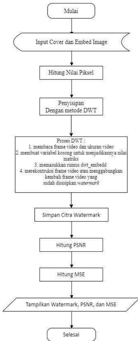
**Gambar 3.6** Flow Chart Proses Penyisipan Metode DWT
