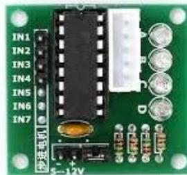
**Gambar 2. 4** Driver Motor ULN2003[12]
