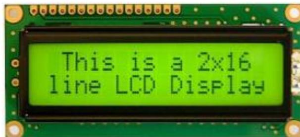
**Gambar 2. 11** Liquid Crystal Display 16x2[21]
