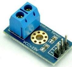
**Gambar 2.8. Voltage sensor**
