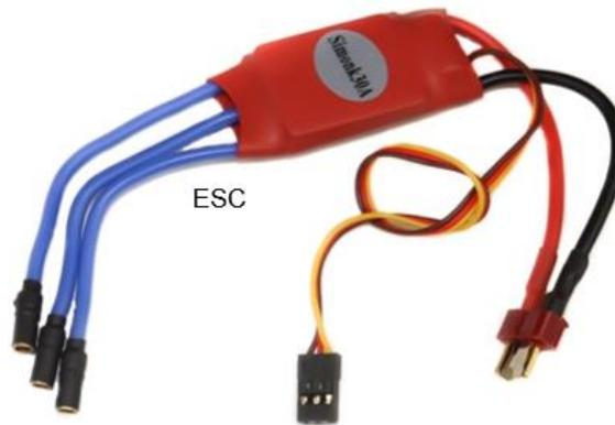
**Gambar 2. 4** *Electronic Speed Control [19].*
