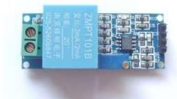
**Gambar 2. 2 Sensor Tegangan ZMPT101b.**
