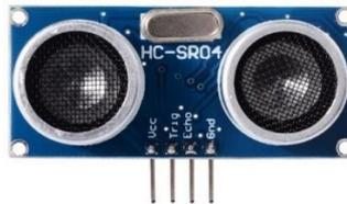
Gambar 2. 5 Sensor Ultrasonik
