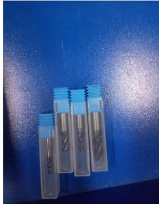
**Gambar 3. 7** Milling Cutter
