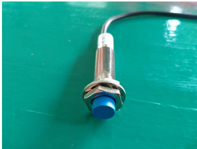
Gambar 2.2. Sensor proximity induktif
