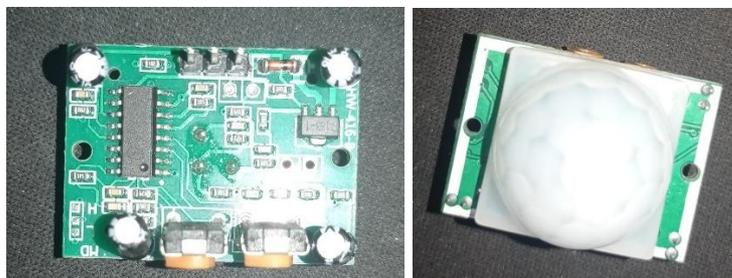
**Gambar 2.6 Sensor Passive Infrared**
