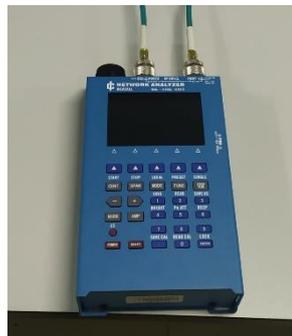
**Gambar 3.6** *Vector Network Analyzer*
