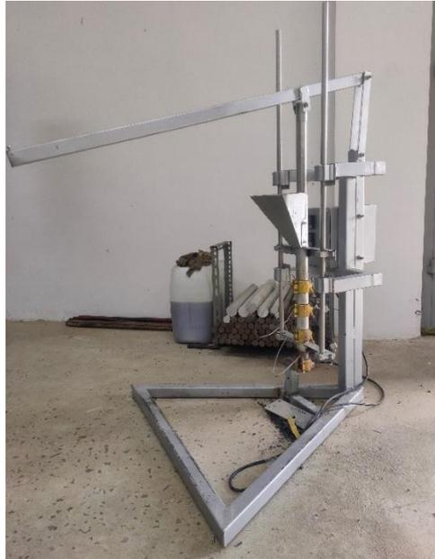
**Gambar 3. 4** *Injection molding tipe plunger*
