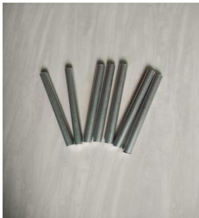
**Gambar 3.14** Batang pin alumunium
