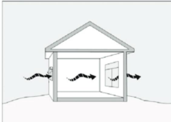
Gambar 47 Sistem *Cross Ventilation*
