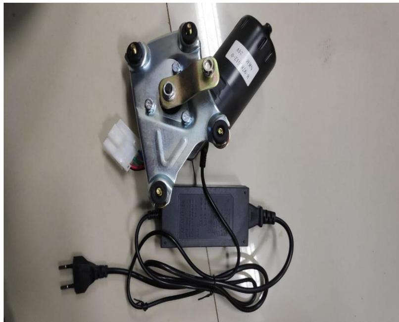
**Gambar 3.3** Motor DC 24 V
