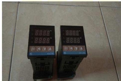
**Gambar 3. 12** *PID Controller*
