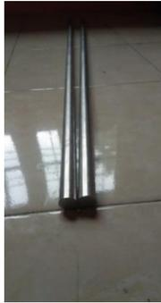
**Gambar 3. 8** Silinder Pejal *Stainlesssteel*, d:16mm
