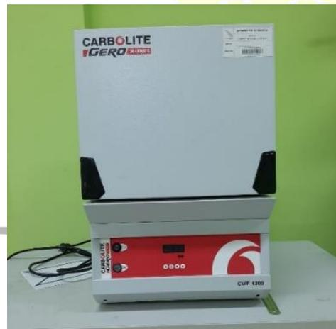
**Gambar 3. 9 Laboratory Chamber Furnace Carbolite CWF 1300.**
