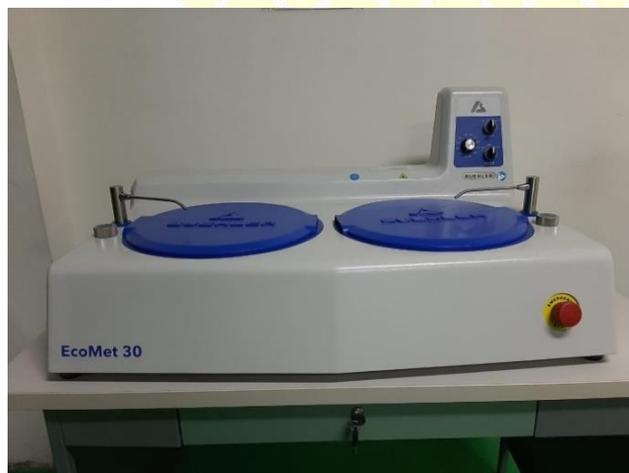
**Gambar 3. 3 Mesin *Polisher Grinder Buehler EcoMet 30 Manual Twin***
