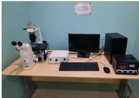
**Gambar 3. 13 Perlengkapan *Trinocular Metalurgical Microscope***
