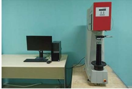
**Gambar 3. 14 Universal Hardness Tester Zwick Roell ZHU 250 CL**
