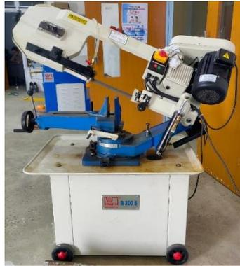
**Gambar 3. 2 Mesin *Band-Saw***
