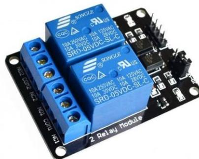
Gambar 2.5 *Relay* dua channel.
