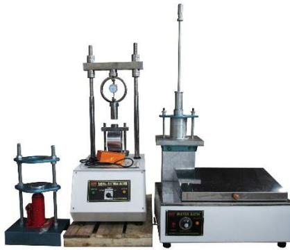
**Gambar 2.8.** Alat uji *Marshall*
