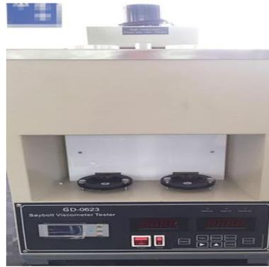
**Gambar 2.7.** Alat Uji Viskositas
