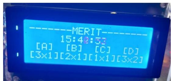
Gambar 29 Tampilan LCD saat *standby mode*
