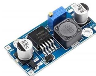
Gambar 11 DC-DC Buck Converter
