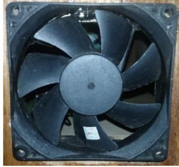
Gambar 2.9. DC Blower FAN  $80 \times 80 \times 25 \text{ mm}^3$ .
