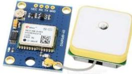
**Gambar 2.5 Modul GPS GY-NEO6MV2**
