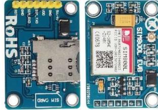
Gambar 2.4 Modul GSM SIM800L V2
