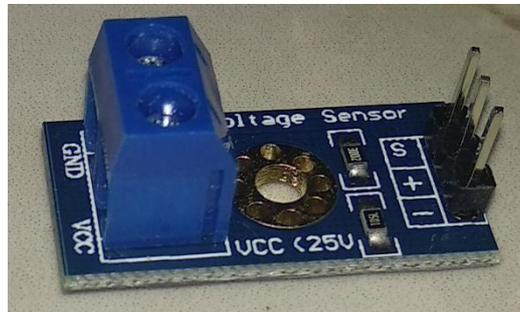
**Gambar 2. 5 Sensor Tegangan DC 25 V**
