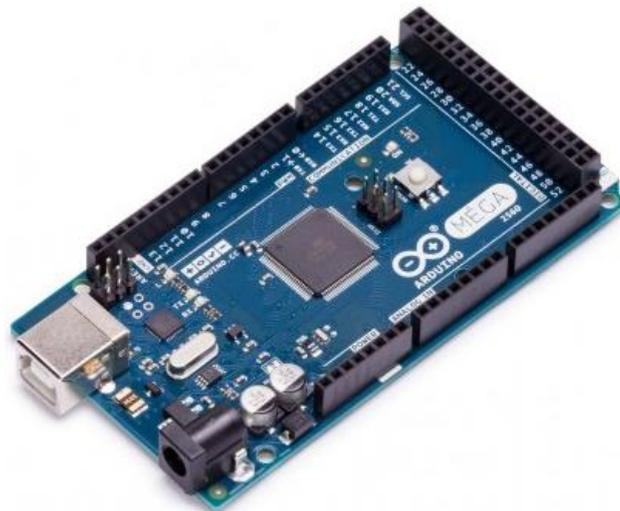
Gambar 2. 9 Arduino Mega2560
