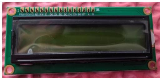
**Gambar 2. 4 LCD 16x2**
