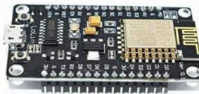
Gambar 3.5 NodeMCU
