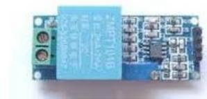
**Gambar 3.2 Sensor Tegangan ZMPT101b**
