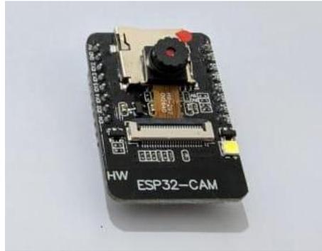
Gambar 2. 2 ESP32 CAM
