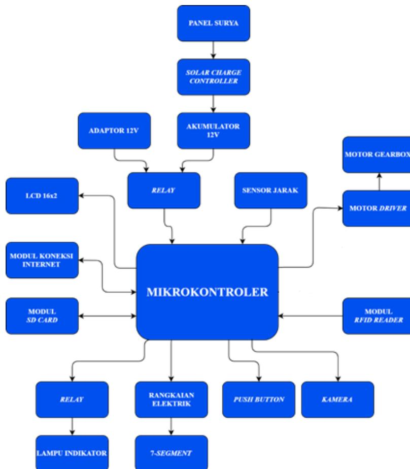
Gambar 3.2. Diagram Sistem Bagian Hardware
