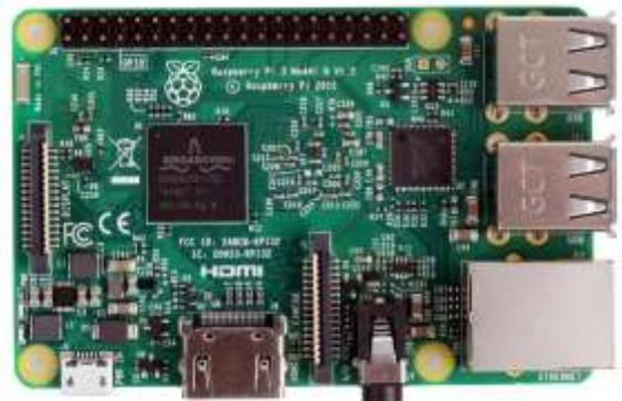
**Gambar 1.** Raspberry Pi 3 Model B+
