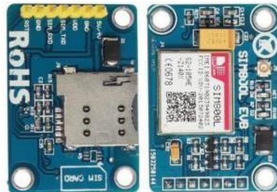
Gambar 2. 3 Modul GSM SIM800L<sup>[8]</sup>.
