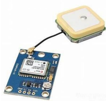
**Gambar 2. 2** Modul GPS *tracker* Neo-6M<sup>[7]</sup>.
