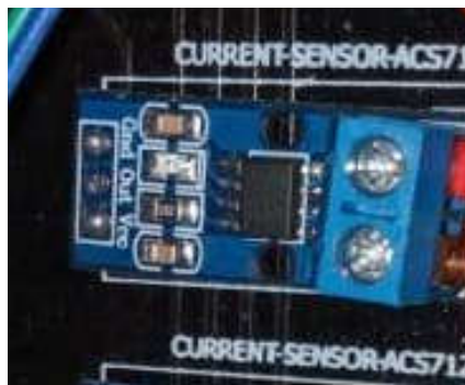
Gambar 3.7 Implementasi Sensor Arus ACS712 5A
