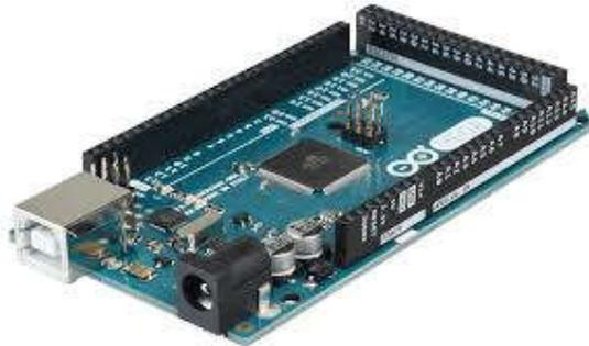
**Gambar 2.6** Mikrokontroler Arduino Mega 2560 R3
