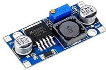
Gambar 11. DC to DC *step down* LM2569
