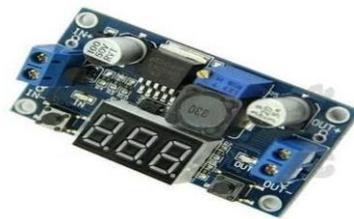
**Gambar 2.15 DC-DC Converter**
