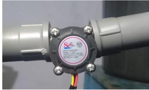
Gambar 2.3 *Water Flow Sensor YF-S201*
