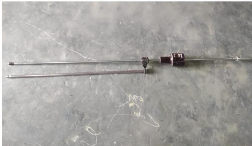
**Gambar 2.9.** Dynamic Cone Penetrometer
