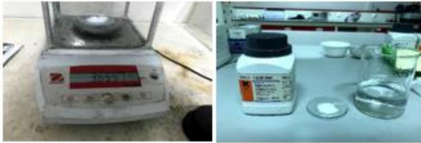
**Gambar 3. 23** Menimbang  $\text{CaCl}_2 \cdot 2\text{H}_2\text{O}$
