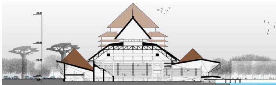
Gambar 2. 6. Potongan Balairung UI Sumber : Kind Architect
