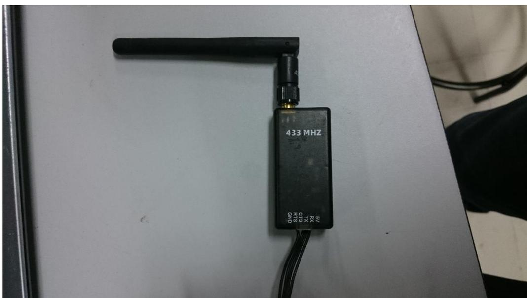
Gambar 3 Modul Radio Telemetry (Radio Frekuensi) 433 MHz
