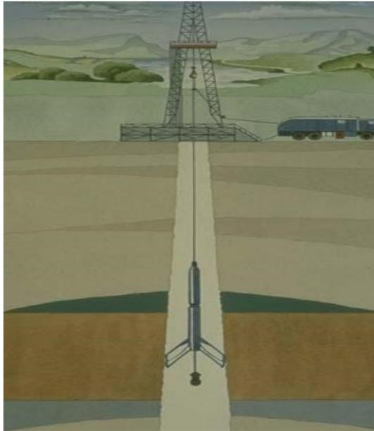
**Gambar 2.9** Pengukuran *well logging* (Darling, 2005)
