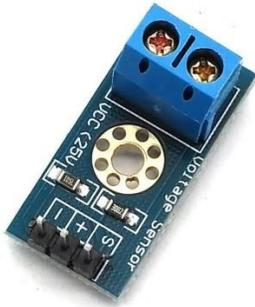
Gambar 4. Sensor Tegangan DC
