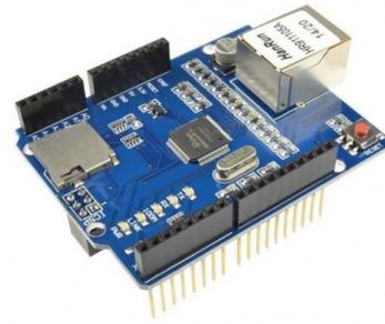
Gambar 2. Ethernet Shield W5100
