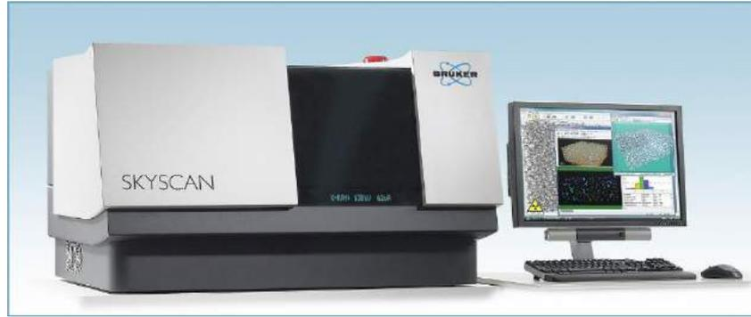
**Gambar 2.1.** Alat  $\mu$ CT-Scan Tipe SkyScan 1173 (FMIPA ITB)
