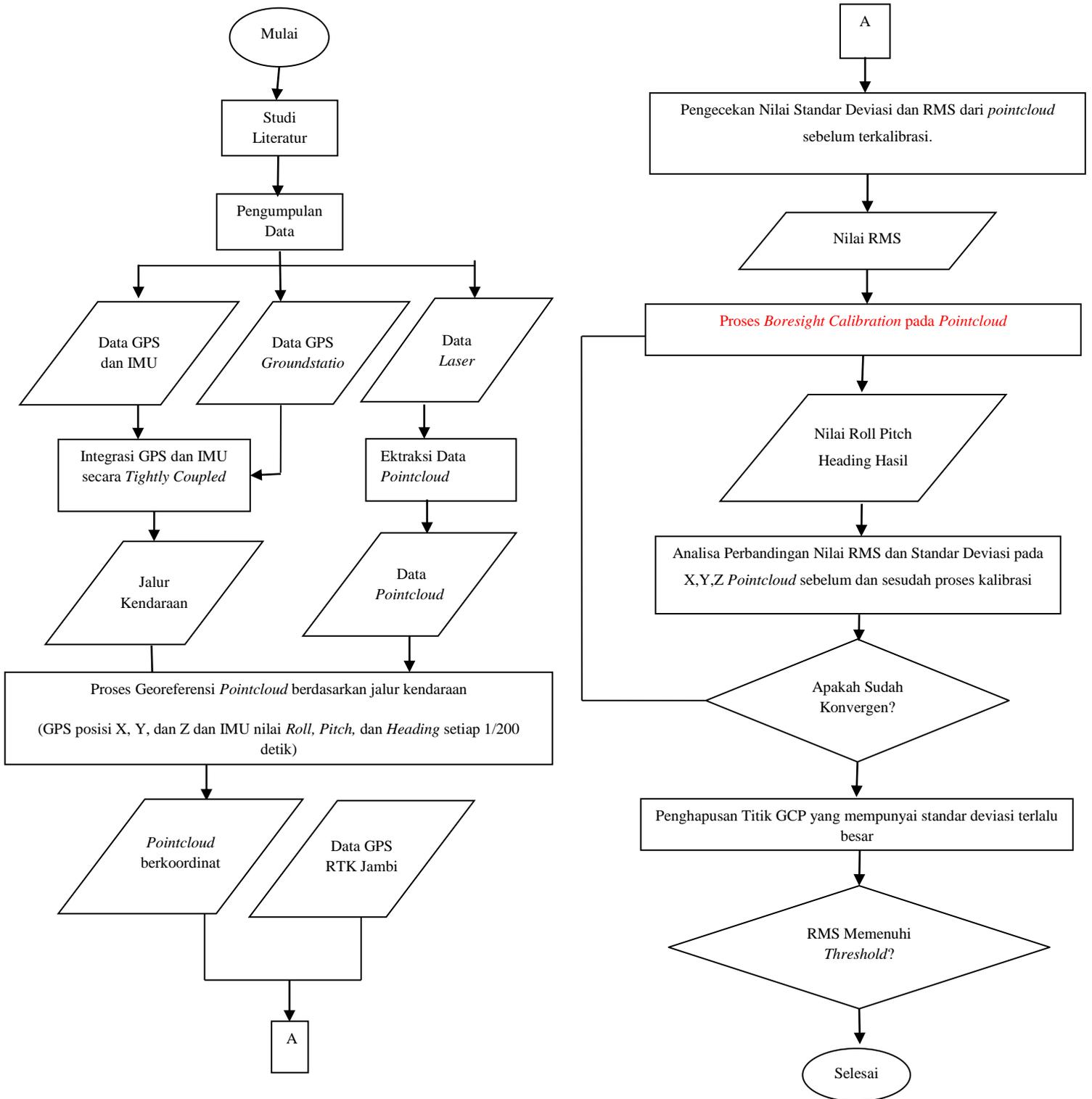
**Gambar 2. Diagram Alir Pengolahan Bore sight Calibration**
