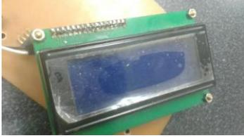
Gambar 6. LCD 20x4
